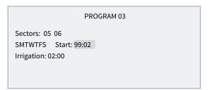
Enter 99 in the two hour digits (indicates that it is sequential) and enter the previous program in the two minute digits. To use 99, it must have been previously configured in 'Function - 4. Parameters - 8. Installer - 5. Various'.
