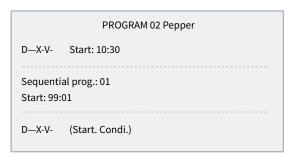
Sectors (<u>00</u> ... 30): sector that will activate the program. There can be up to 4 sectors as configured in 'Function -4. Parameters - 10. Installer - 5. Various'. If they are all 0, the program is inactive.
