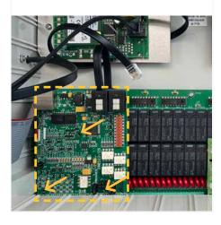
7 Separate the keyboard part of the box by carefully pulling the flat gray tape that joins the two plates, then replace it with the new Agrónic 4500 front.
