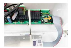
8 If the unit has the analog I/O board, install it again as it was removed in step 6.
