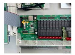
8 If the unit has the analog I/O board, install it again as it was removed in step 6.
