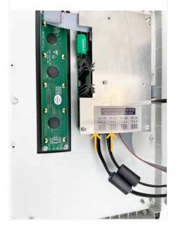
**2** Remove the six side screws and two central screws.
