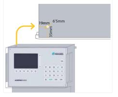
Close the unit and replace the four screws removed in step 2.
