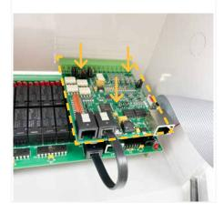
7 Separate the keyboard part of the box by carefully pulling the flat gray tape that joins the two plates, and replace it with the new Agrónic 4500 front.
