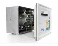
6 If the Agrónic 4500 unit has an analog I/O option, remove the option by removing the three screws, so that the front can be changed.
