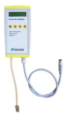
Transmitters generally come factory-configured. However, it is possible to perform consultations or configurations by using a "Module Reader," consisting of a screen and four keys, which connects to the transmitter through the only visible connector on the inside.
