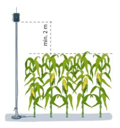
To increase the coverage, and if necessary, the best system is made by raising the module as high as the length of the cable allows.
