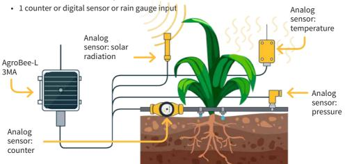
As an example, the 4-20mA sensors that this model manages can record temperature, pressure, trunk/fruit dilation, wind, radiation, etc.
