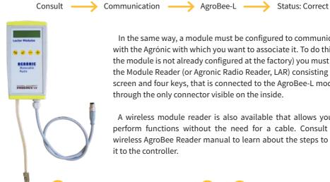
In the same way, a module must be configured to communicate with the Agrónic with which you want to associate it. To do this (if the module is not already configured at the factory) you must use the Module Reader (or Agronic Radio Reader, LAR) consisting of a screen and four keys, that is connected to the AgroBee-L module through the only connector visible on the inside.
