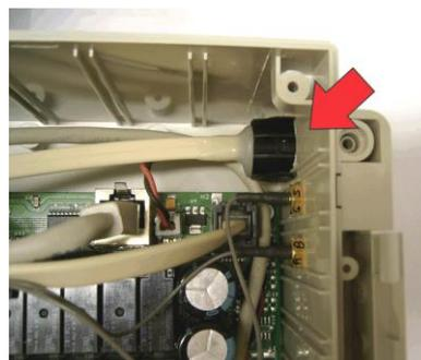
Phone jack must be connected to the H10 connector that is placed in the board behind the keyboard. Look at the following picture.
