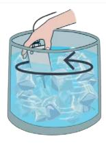
4 Stir until temperature is stable around 0°C.
