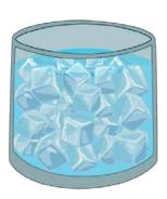
Stir the ice and water mixture for two minutes so that water temperature reaches the melting point of 0°C.
