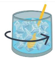
3 Insert the sensor halfway and stir the ice and water mixture steadily for some minutes.
