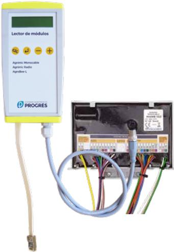
You can configure the MAM with the Module Reader, consisting of a screen and four keys. It is not necessary to deactivate the MAM before connecting it.
